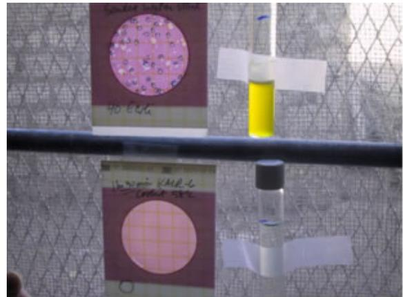
**Fig. 4** Petrifilm (left) and Colilert MPN tube (right) tests of Meatu water before and after heating in Cookit. E. coli.= Blue colonies with gas on Petrifilm. Fluorescence of Colilert tube indicates the presence of E. coli.
