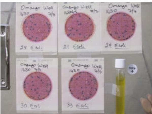
**Fig. 8 Results of water from shallow well in Nyakach, heavily contaminated with E. coli, and a danger to health.**
