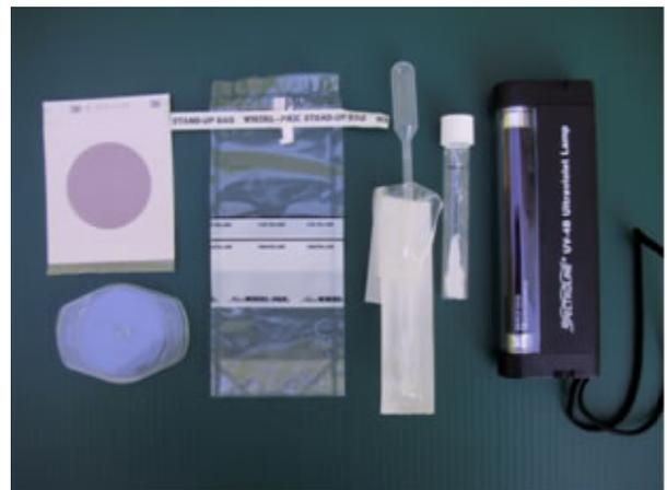
**Fig. 11 Items used in portable microbiology lab. Petrifilm and spreader, WhirlPak, sterile pipette, Colilert, portable UV light.**
