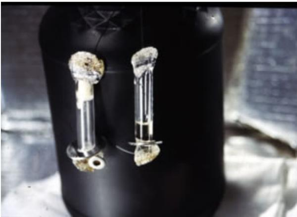
**Fig. 2** Water Pasteurization Indicator. When water heats to 65°C, the wax melts and falls to the bottom of the WAPI, indicating the water has been pasteurized.
