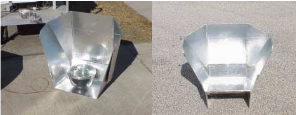
Figure 6 FSEC/High Back solar cooker (Note that the cooker on the right has the front reflector)
