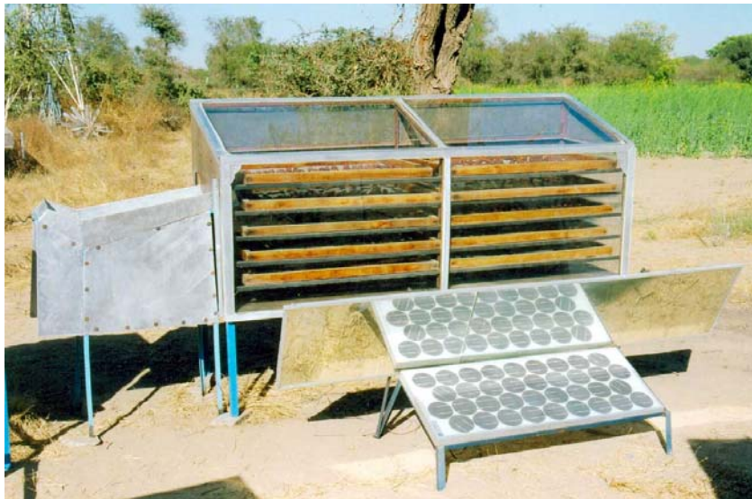
Fig.2 b. PV dryer with PV panel and reflector of extended length used for drying ber
