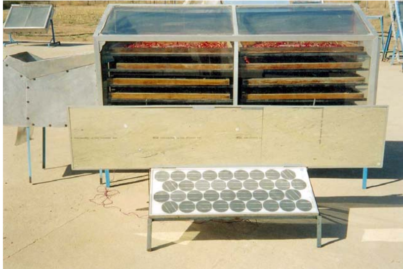
Fig. 3. Drying of Chillies in PV dryer with winnower's fan
