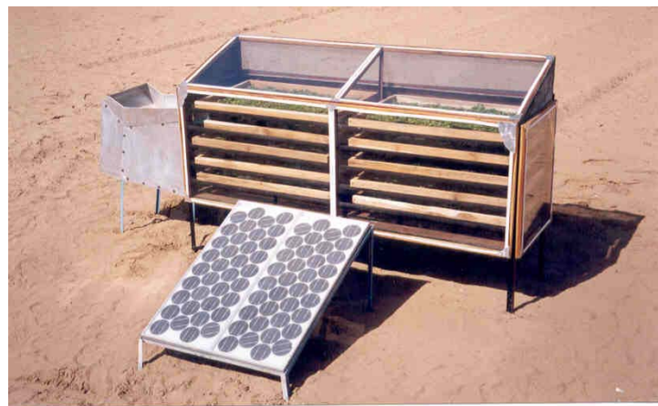
Fig. 1.b PV winnower added to dryer (Drying of coriander leaves)
