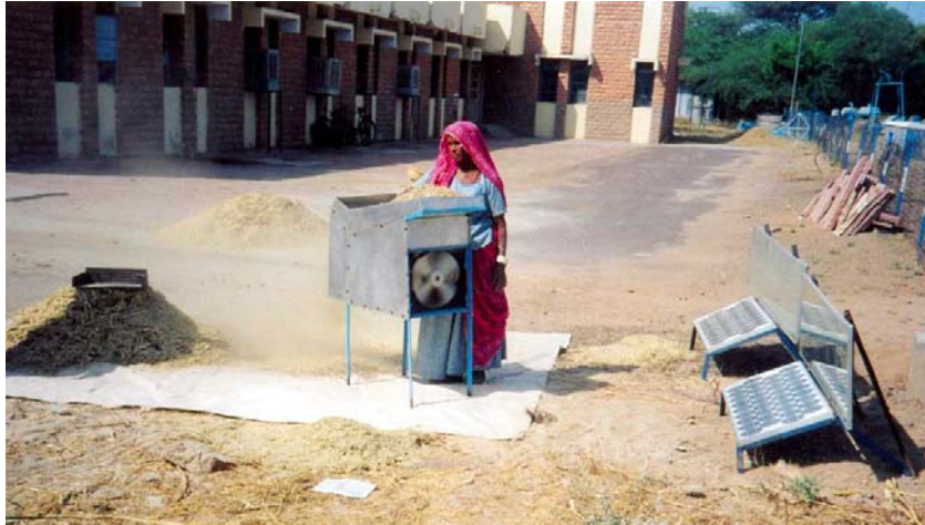
Fig.2 a. PV winnower with single PV module and reflector of extended length
