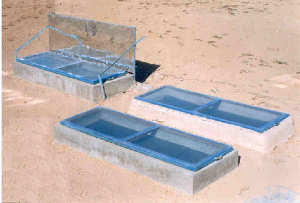
Fig.1 Animal feed solar cookers made of vermiculite cement and clay etc.
