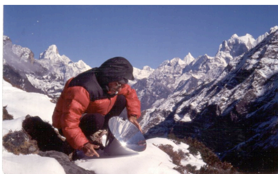
Fig.4 Solar Backpack “Trekking” Cooker (made by FAST) preparing food or melting snow for drinking
