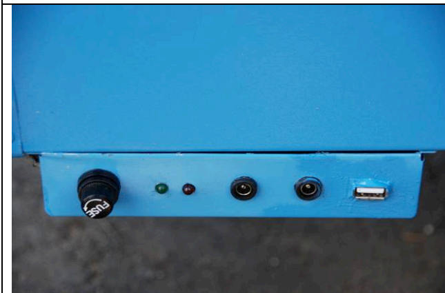
This is the electricity panel with the fuse (left), 2 plugs for light and radio and a USB point to charge mobile telephones
