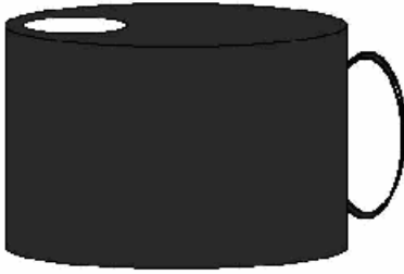
Figure 13 Shows a special tea pot for Solar Picnic, which is built from 500 ml tomato juice can. Once given the proper shape of long ellipsoidal cross section, its capacity is reduced to 300 ml.
